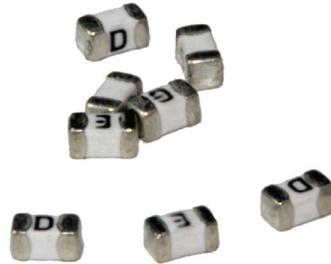
AEM's SolidMatrix® is offered in EIA 0402, 0603 and 1206 case sizes with Fast Acting, Slow Blow and High In-rush series. From 0.5A to 30A current rating and 24VDC and 64VDC voltage rating, AEM's SolidMatrix® provides excellent secondary overcurrent protection for DC power applications.
